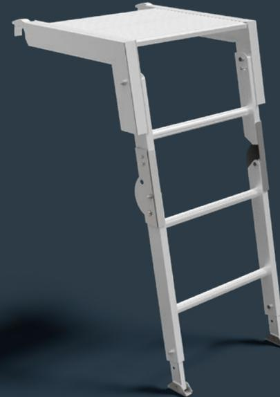
The Alto Scaffmate Duo has the added flexibility of 2 working platform heights. Unlock the lower half of the ladder and fold away to use the Scaffmate for 0.5m heights, removing the need for carrying 2 types of hop-up components.
